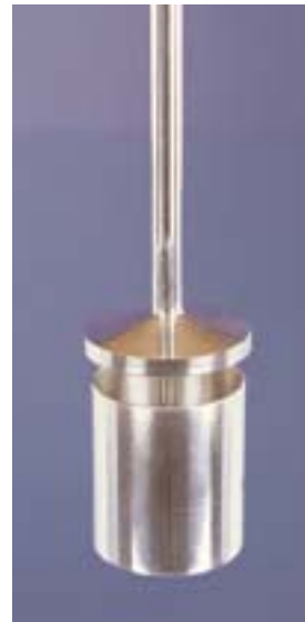
Liquid Cup Sampler - single hand operation
