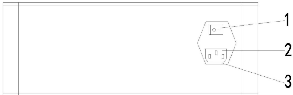
Figure 2: The rear view of the Block Heater. 1, on/off switch; 2, IEC power inlet; 3, fuse holder
